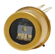
The CPOD serials cooled InAsSb photodiode is a photovltaic muti-junction device that provides reduced noise for detecting mid-infrared light in the 2.2-6.6 µm range. These detectors are integrated with one stage TEC cooler and hermetically sealed to ensure longevity. It has an AR coated silicon window and package in a TO39 can. It is fully compliant with RoHs. Additionally, a driving PCB with an amplifier is available for convenient use.
